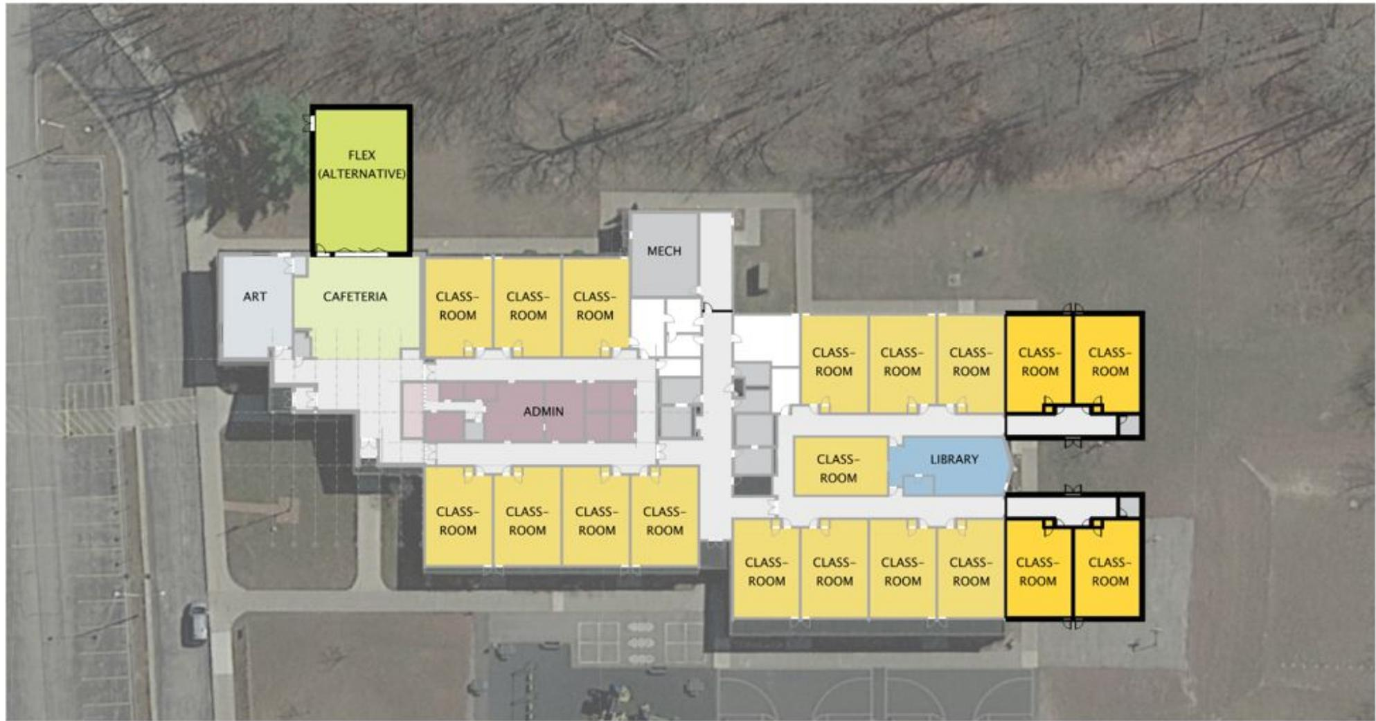
FIRST FLOOR PLAN - 5,000 SF BASE / 2,100 SF ALTERNATE
